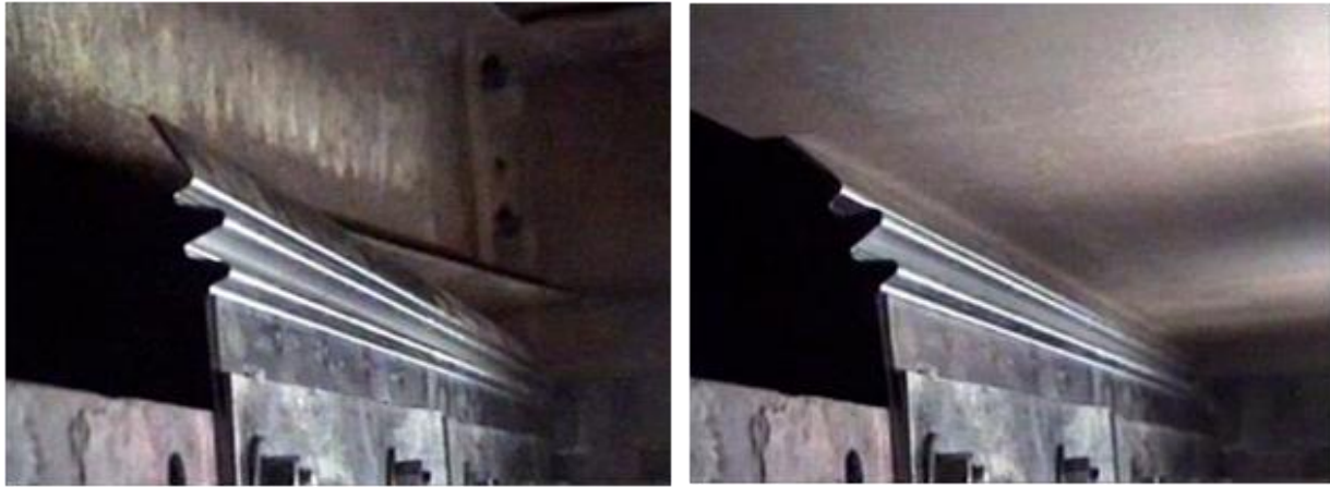
Figure 12, Continuous Contact DURAMAX Seal (before & after sector plate contact)
