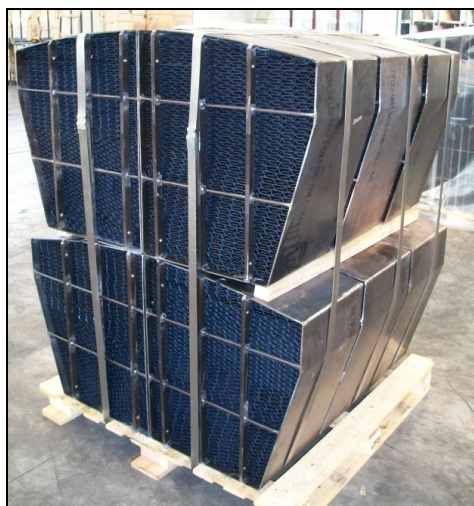
Figure 12: Vitreous Enamel Coated elements/baskets supplied to HECO, Kahe Point
