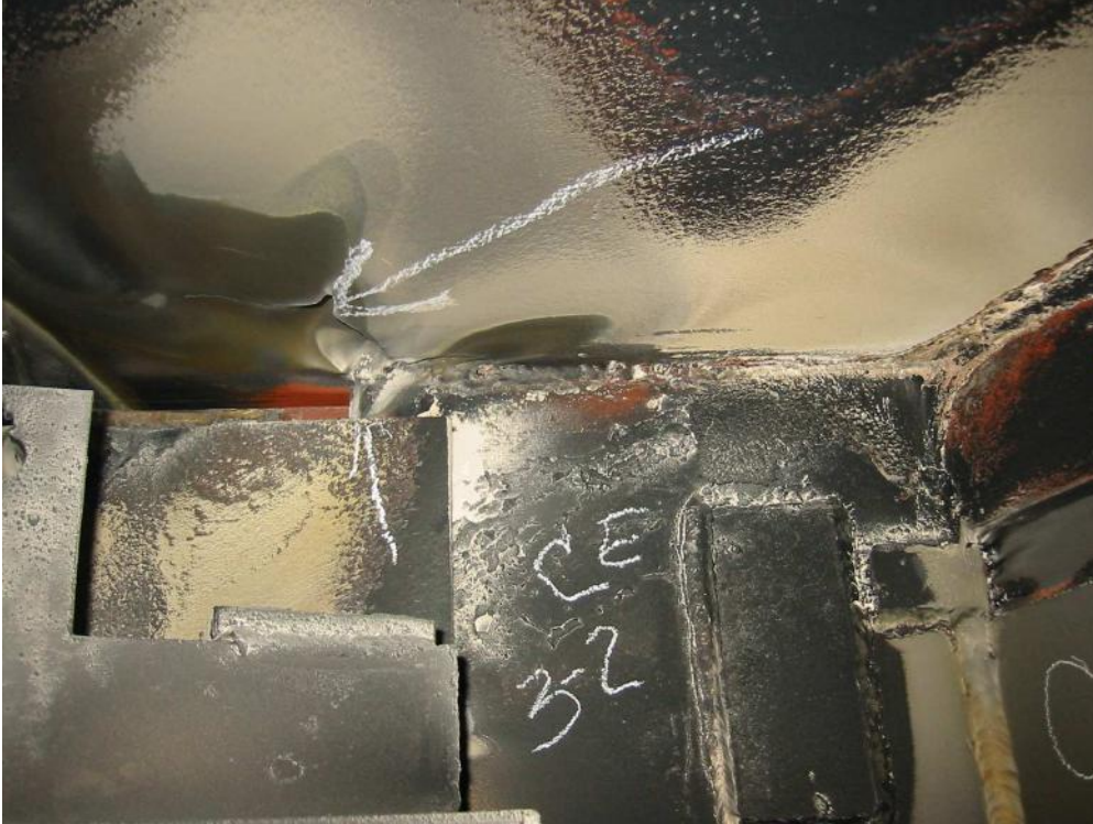
Cold end spool erosion damage
