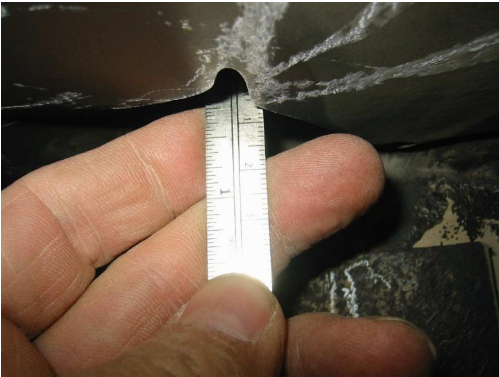
Cold end spool erosion damage
